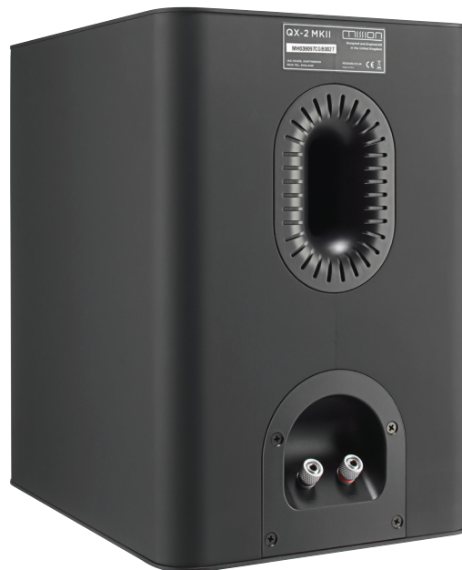
An unusual rear port with serrations to improve air flow, Mission say. Tuned to 40Hz it also helps the small 'speaker go low – right down to 30Hz our measurements show. One pair of terminals is fitted for mono-wiring; they accept 4mm banana plugs, bare wires or spades.
