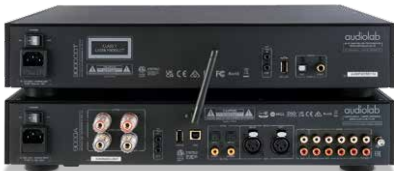
ABOVE: CD transport [top] has opt/coax digital outs and a USB-A port for 44.1/48kHz media on an external drive. Amp [below] has MM, three line ins, a power amp in and pre out on RCAs plus 2x coax/opt digital inputs, a USB-B (768kHz/DSD512) input and main outputs on 4mm speaker binding posts
